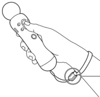
Use the strap lock to tighten the strap.
