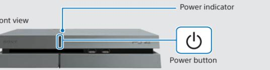
If video is not displayed on the screen or video is not correctly displayed when the system is turned on (the power indicator lights up in [ ] white), touch the (power) button for at least 7 seconds (until the system beeps a second time) to turn off the power, and then turn on the power again.
