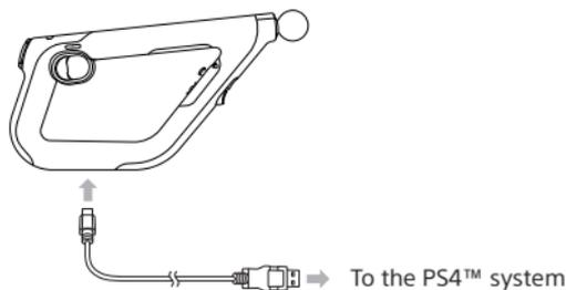
The sphere flashes slowly when charging, and stops flashing when charging is complete.
