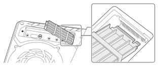
5 Tilt the M.2 SSD down and fasten it with the screw.
