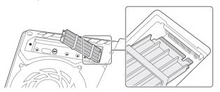
5 Tilt the M.2 SSD down and fasten it with the screw.
