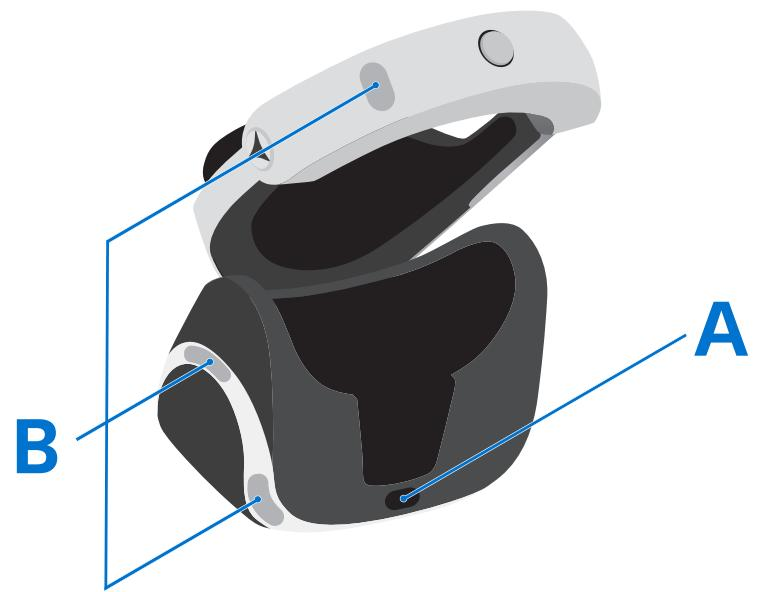
To turn off your VR headset, press the ⚡ (power) button (A) until you hear a beep. The tracking lights (B) will turn off.
