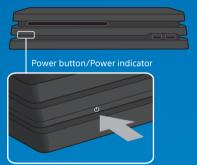
If your TV does not display a picture when the power indicator turns white, restart your system. Press the  $\bigcirc$  (power) button for at least 7 seconds to turn off your system, and then turn it on again.
