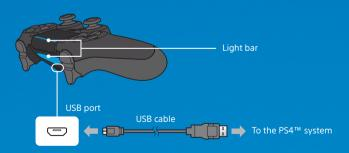
To charge your controller while your system is in rest mode, select an option other than [Off] in (Settings) > [Power Saving Settings] > [Set Features Available in Rest Mode] > [Supply Power to USB Ports].
