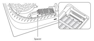
(3) Tilt the M.2 SSD down and fasten it with screws.
